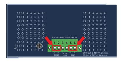
2. Tighten the wire-clamp screws for preventing the wires from loosening.
